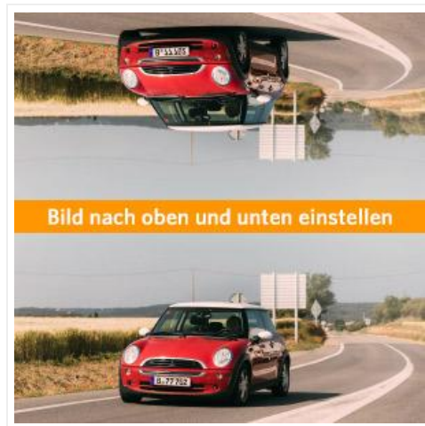
Figure 4.3: The image can be adjusted vertically (up and down) through the menu, providing flexibility for various mounting positions, such as below the license plate.
