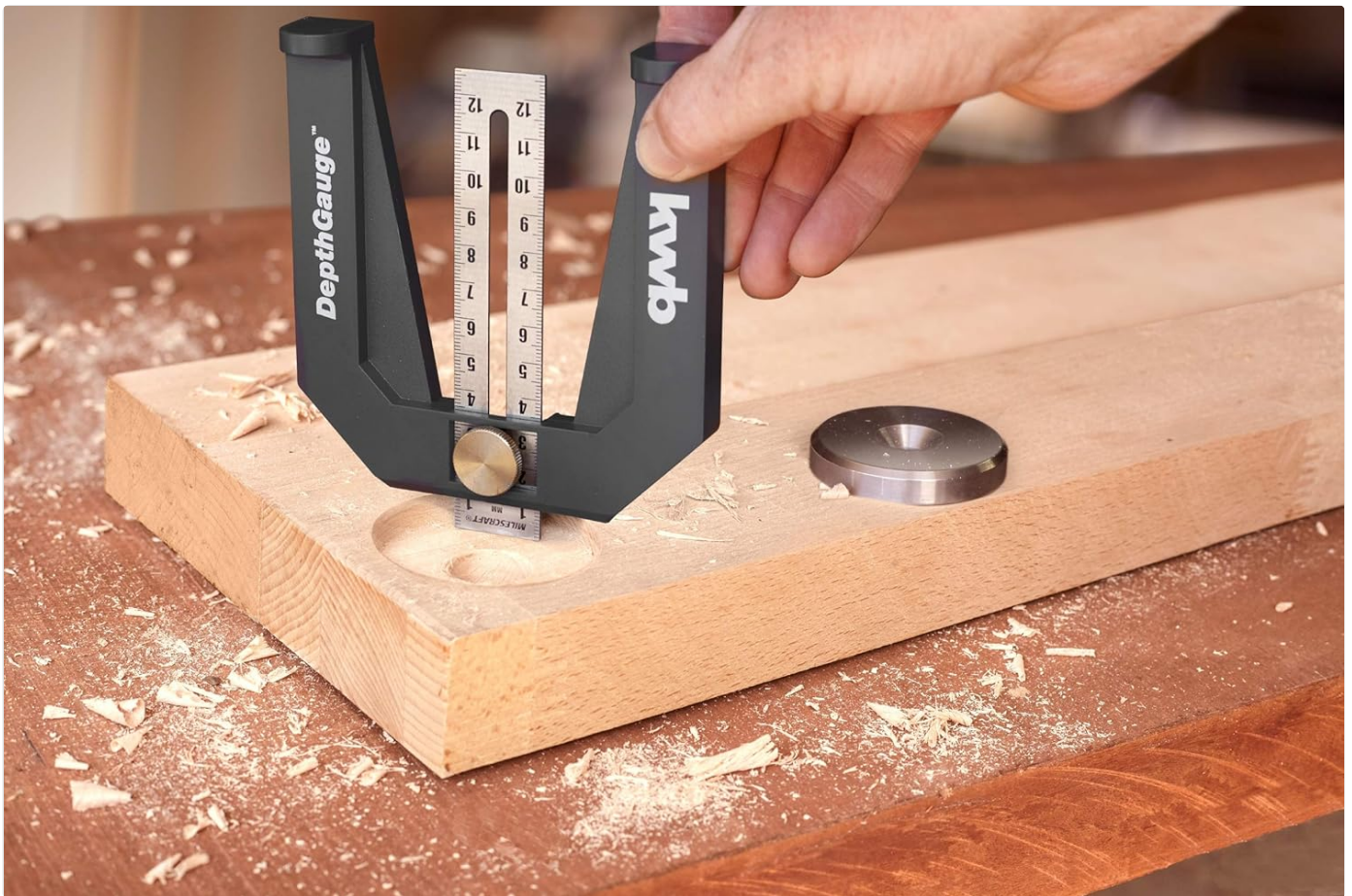
Figure 3: Demonstrating the use of the depth gauge to measure the depth of a routed groove in a wooden workpiece.
