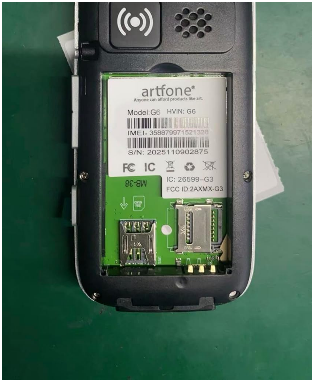
Figure 3.3: Rear view of the artfone S401 with the battery cover removed, exposing the battery compartment, SIM card slot, and microSD card slot for memory expansion.
