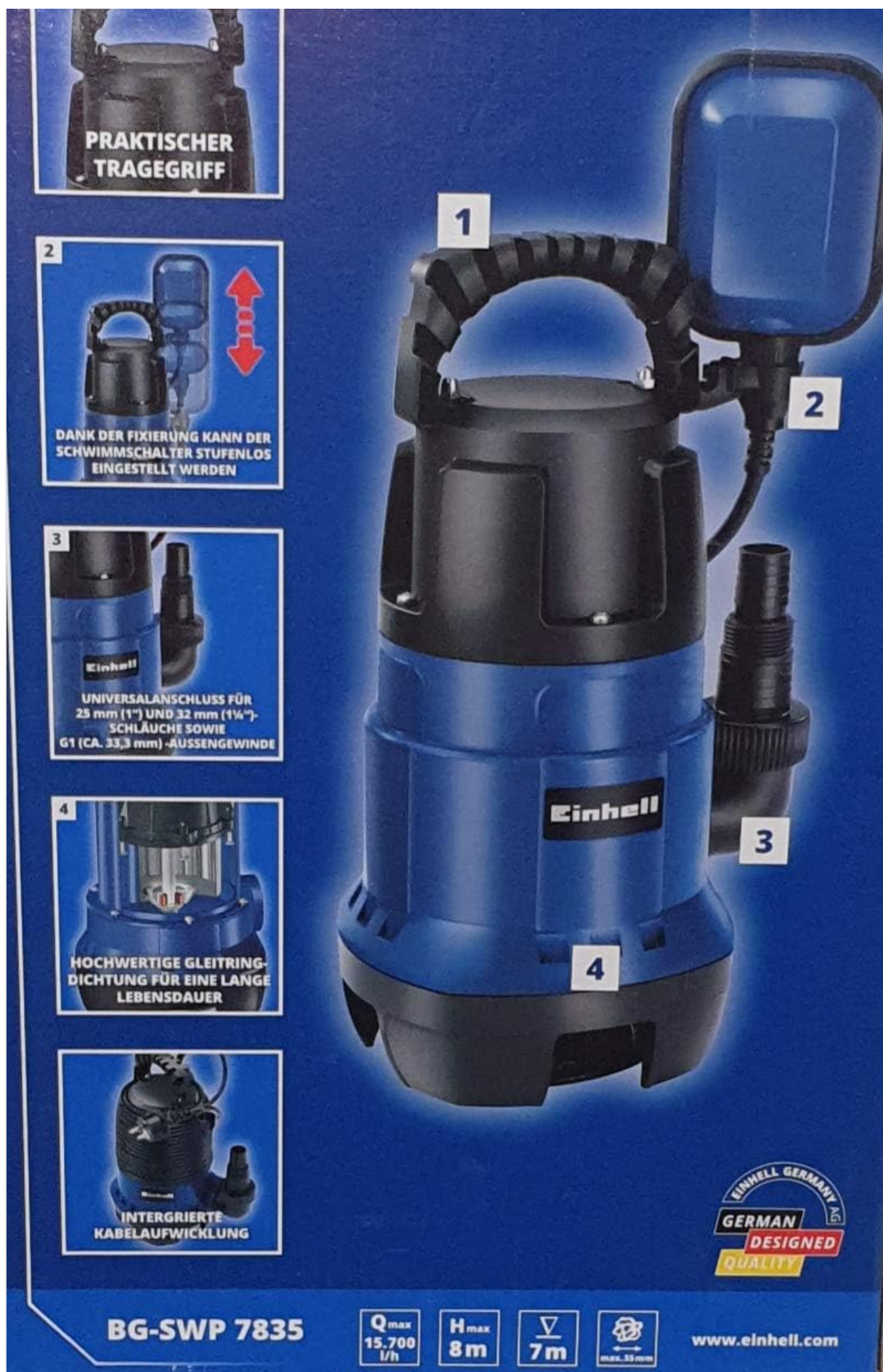
Image 2: Key components of the Einhell BG-SWP 7835 Dirty Water Pump. This image illustrates the pump with numbered callouts pointing to its main features: 1. Practical carrying handle, 2. Height-adjustable float switch for automatic on/off control, 3. Universal hose connection for 25/32 mm hoses and G1 external thread, and 4. High-quality ceramic/rubber mechanical seal for durability.
