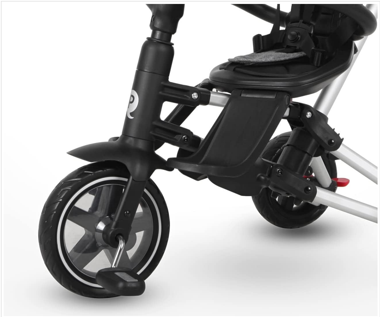
Figure 4.1: A close-up of the front wheel and non-slip pedals, illustrating the mechanism for child-powered movement.
