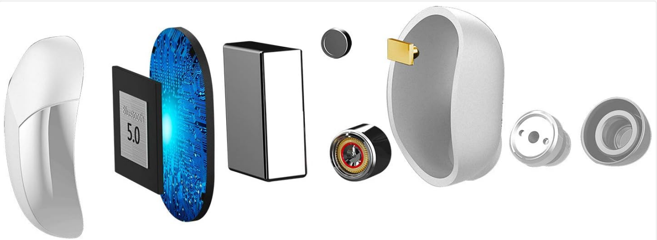
Image 3.3: An exploded view illustrating the internal components of a Celly FLIP1 earbud, including the Bluetooth 5.0 chip, battery, and speaker driver.
