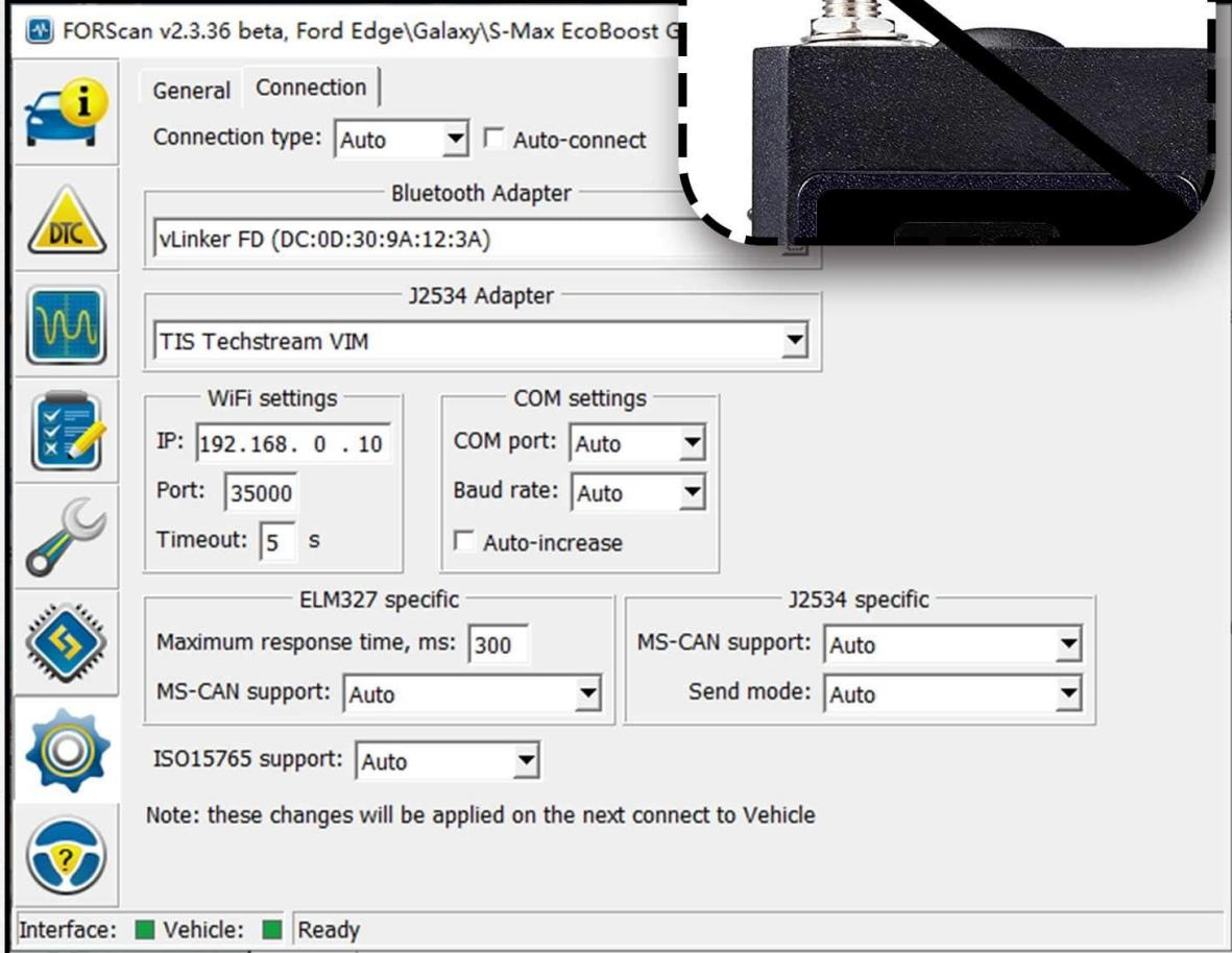
A screenshot of the FORScan Windows interface demonstrating the automatic network switching feature, eliminating the need for a physical toggle switch.
