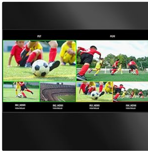
Figure 6: The multi-view display showing four input sources, with the Program (PGM) and Preview (PVW) outputs highlighted.
