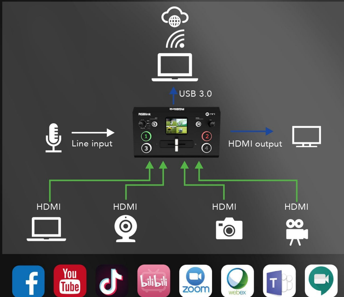
Figure 3: Diagram illustrating the connection of HDMI inputs, line input, USB 3.0 output to a computer, and HDMI output to a display.
