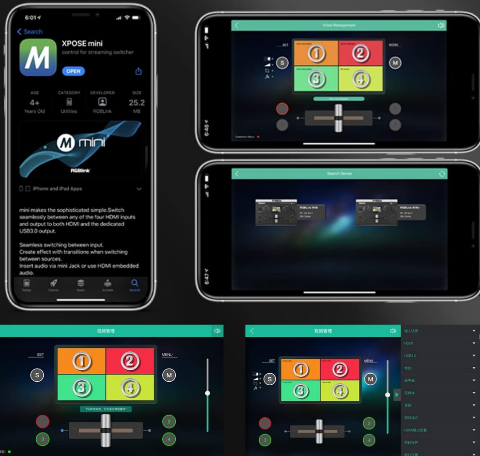
Figure 9: Screenshots of the RGBlink control application interface on a smartphone, demonstrating remote control capabilities for the switcher.
