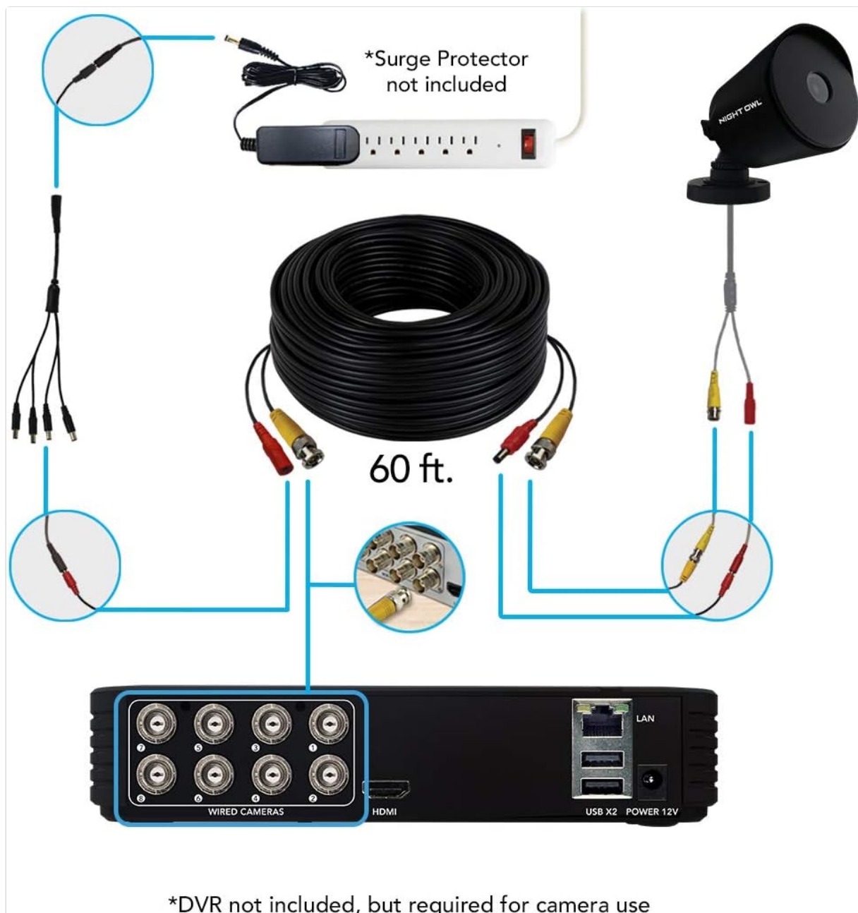
Image 1.1: Included components: two Night Owl cameras and two 60 ft video/power cables.
