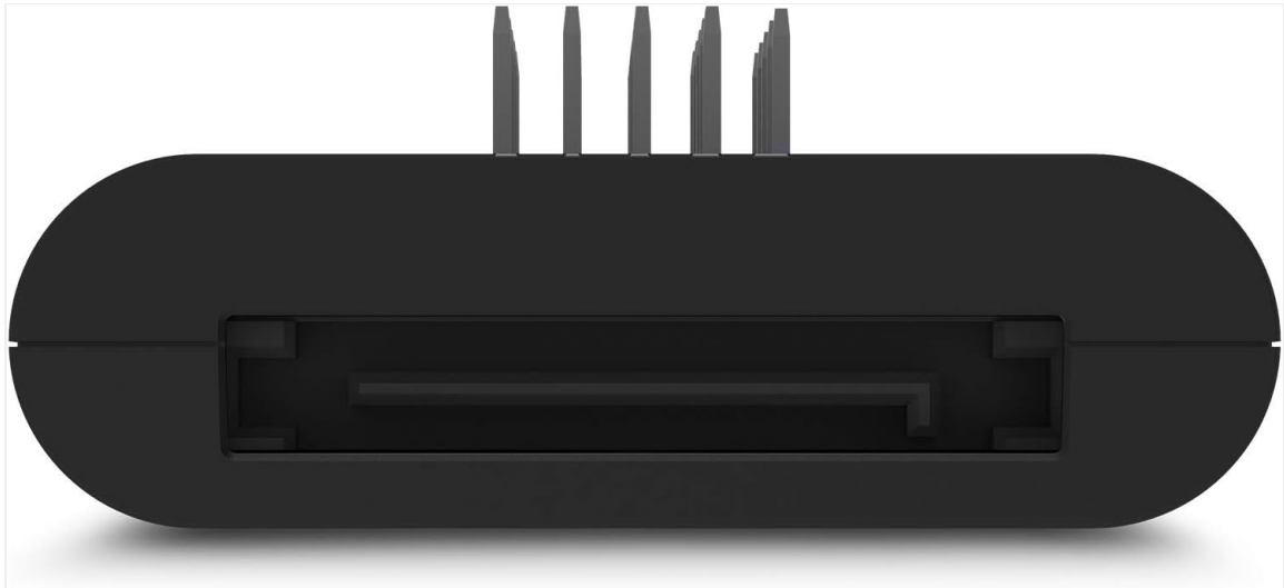
Figure 4.1: Side view of the hub, highlighting the SATA power connection port.
