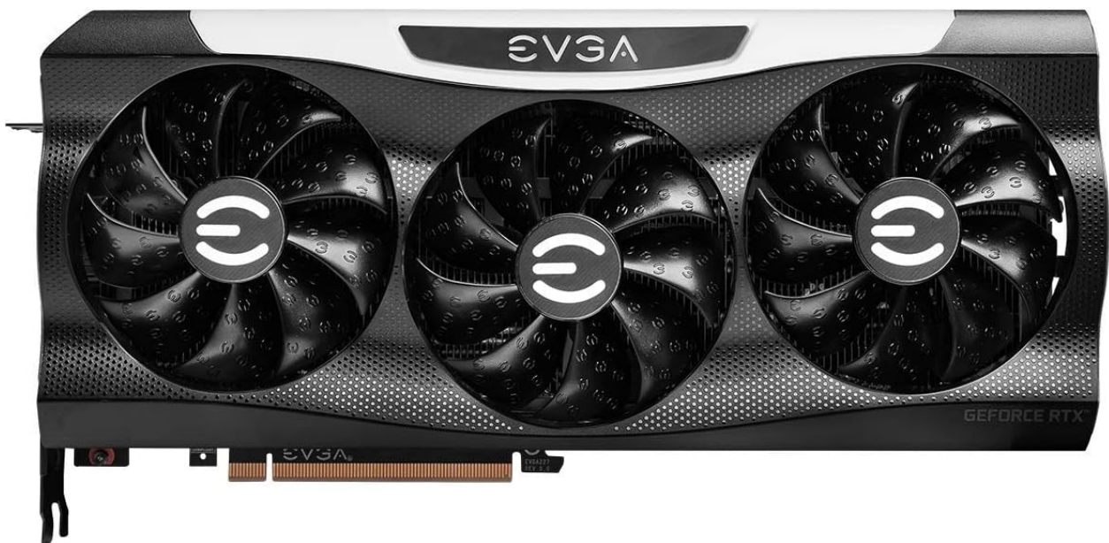
Figure 3: Front view of the graphics card, showcasing the triple fan design.
