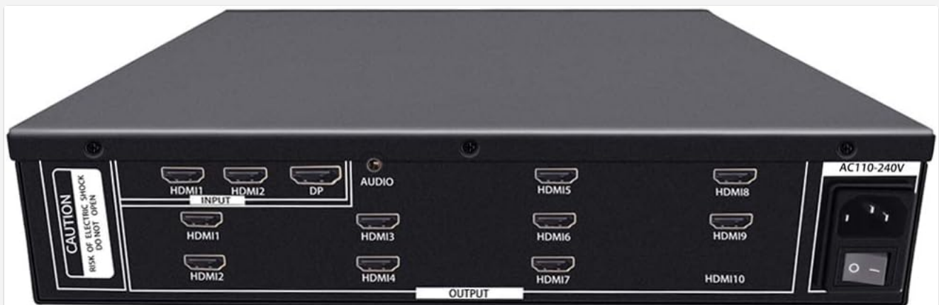
Figure 3: Rear Panel. The rear panel of the ISEEVY ISV-TWC9-4K60 Video Wall Controller, displaying multiple HDMI input ports (HDMI1, HDMI2), a DisplayPort (DP) input, an Audio output (3.5mm jack), nine HDMI output ports (HDMI1-HDMI9), and an AC power input with a power switch.
