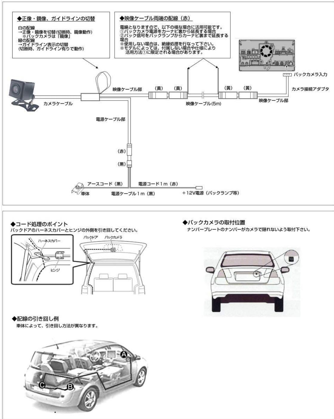
**Image:** Comprehensive wiring diagram detailing the connections for the camera, including power, video, and the white/green wires for image orientation and guideline control. Also shows recommended cable routing and mounting positions.
