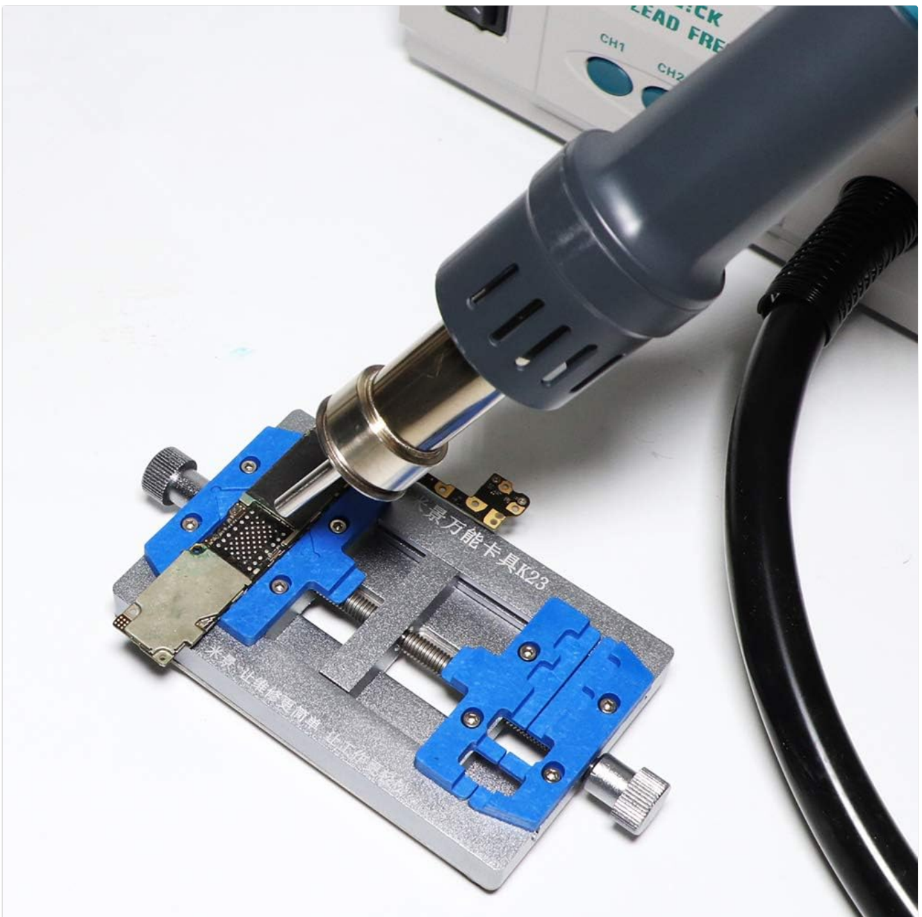
Figure 6: Hot air gun in use for desoldering a chip on a PCB.
