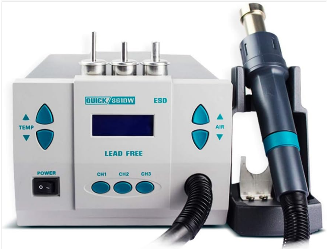
Figure 2: Front view of the Quick 861DW station showing the control panel, display, and hot air gun with nozzles.
