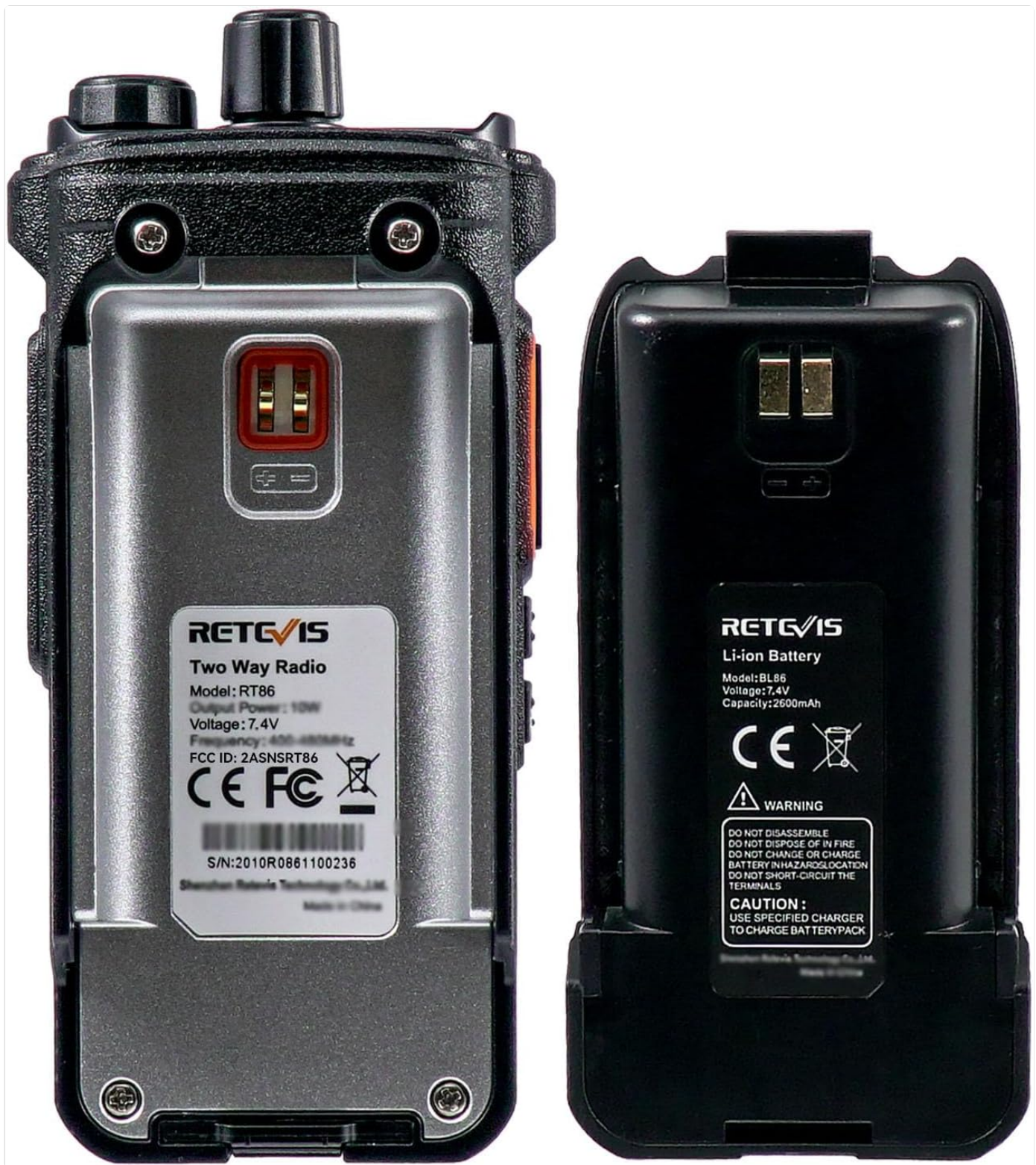
Figure 5.1: The back of the RT86 radio and its removable 2600mAh Li-ion battery.
