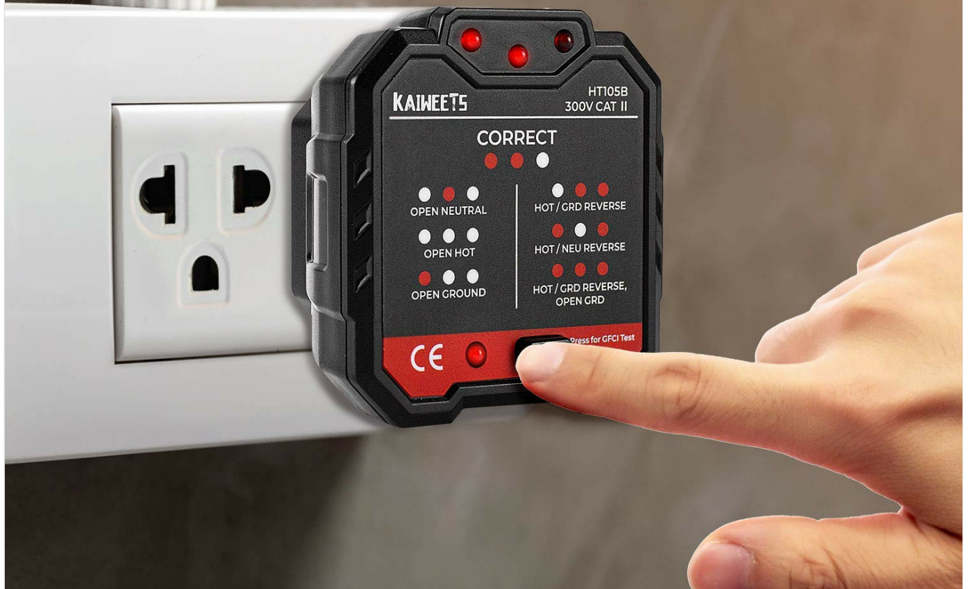
Figure 5.6: Pressing the GFCI test button on the outlet tester.
