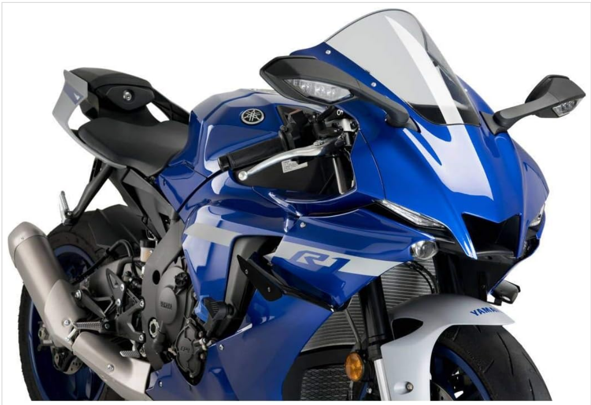
Figure 1: Puig Downforce Spoilers mounted on a Yamaha YZF-R1/M. This image illustrates the spoilers integrated into the motorcycle's side fairings, enhancing its aerodynamic profile.
