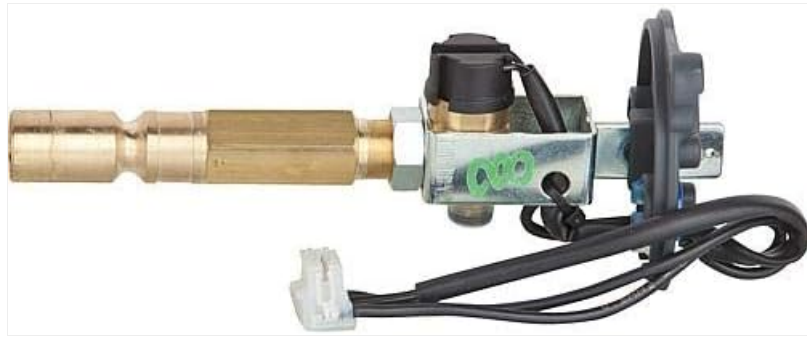
Figure 1: Side view of the Riello RG1R 3007656 Nozzle Assembly. This image shows the brass nozzle body, the electrical connections for the preheater and thermostat, and the mounting bracket.
