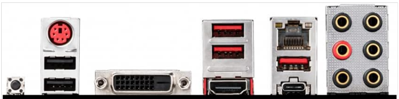
Figure 3.3: Rear I/O panel of the MSI B450 TOMAHAWK MAX II Motherboard, showing USB ports, HDMI, DVI-D, LAN, and audio jacks.
