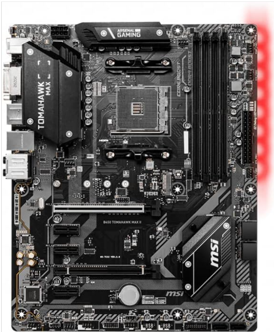
Figure 3.2: Top-down view of the MSI B450 TOMAHAWK MAX II Motherboard, highlighting the CPU socket, DIMM slots, PCIe slots, and various headers.
