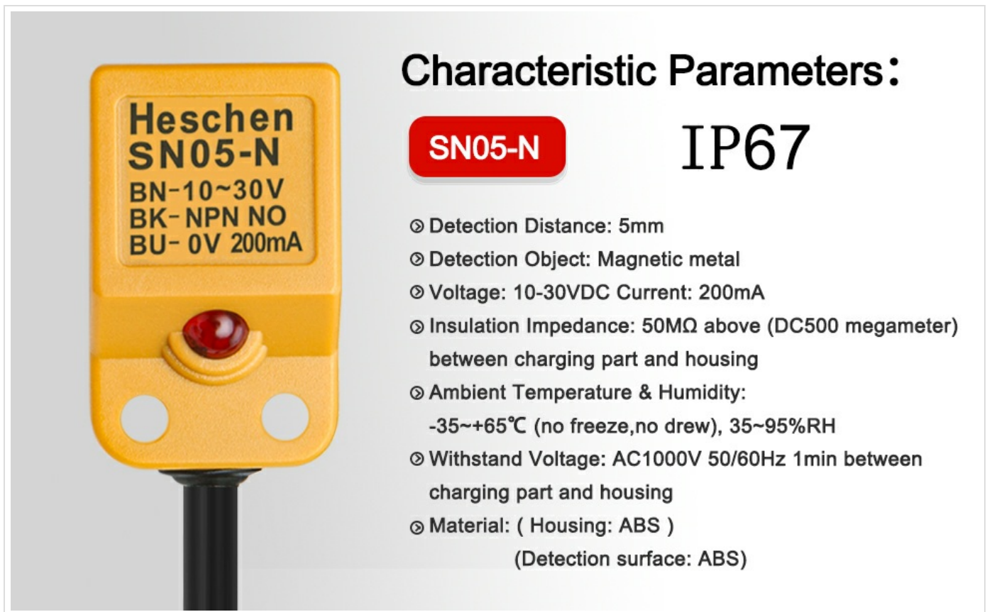
Image 2.2: Visual representation of key characteristic parameters including IP67 rating.
