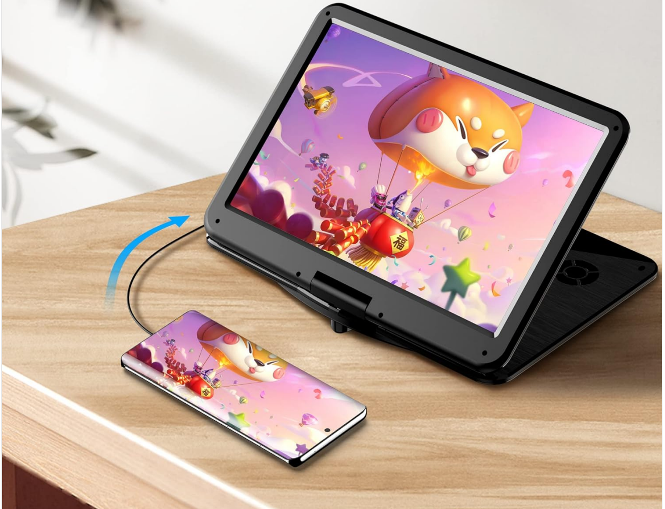
Figure 4: The portable DVD player receiving input via its HDMI port from a smartphone.
