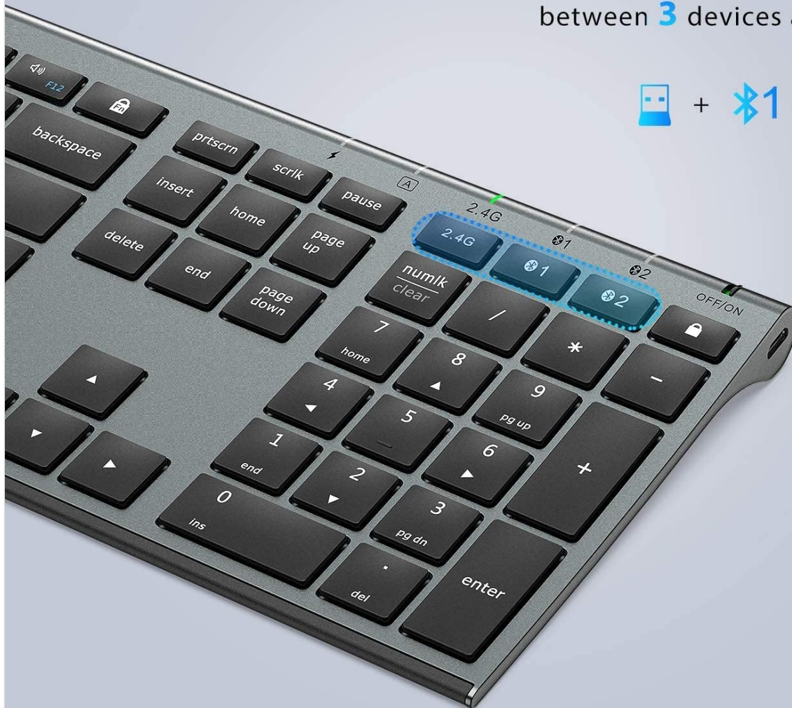
Image: Close-up of the iClever keyboard showing the 2.4G, BT1, and BT2 channel selection buttons.
