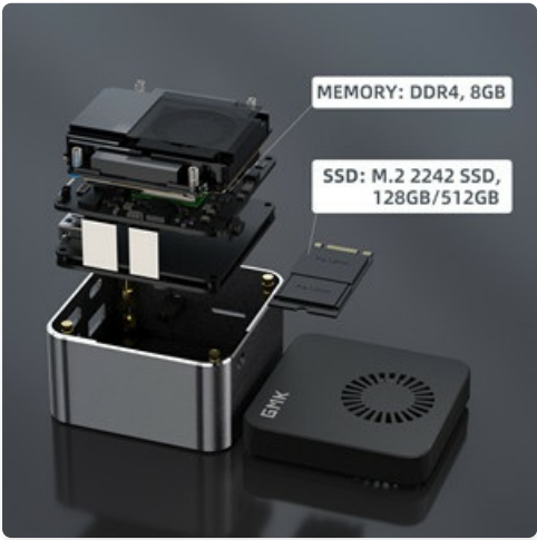
Figure 4: An exploded view of the NucBox KB1, illustrating the internal DDR4 8GB memory and the M.2 2242 SSD (128GB/512GB options), which can be upgraded.
