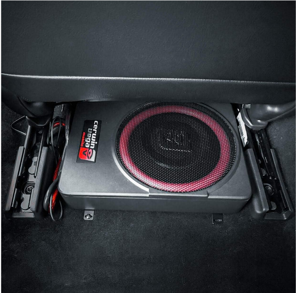
Image 5.1: The VPAS10v2 subwoofer shown installed discreetly under a vehicle seat, demonstrating its low-profile design.
