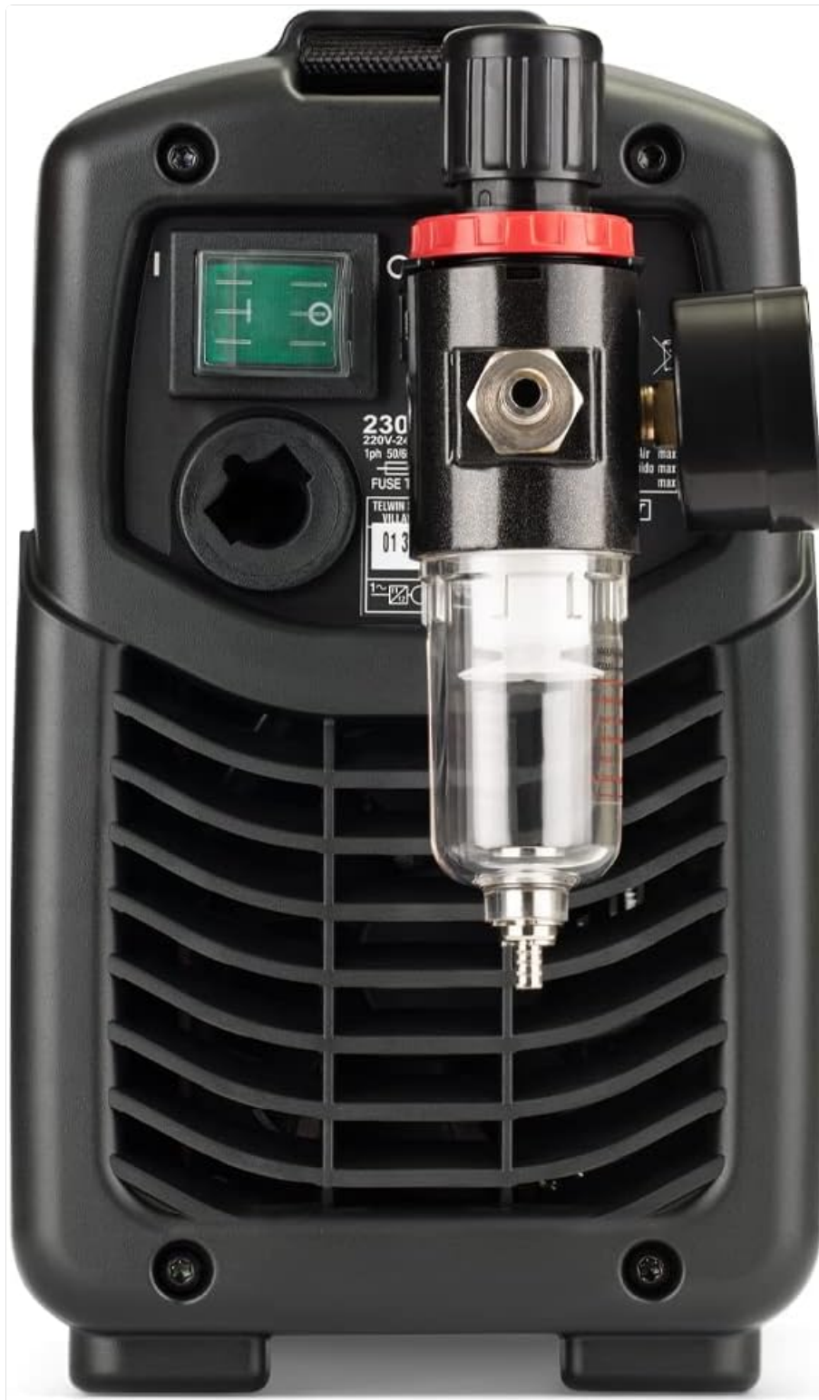
Figure 3.3: Rear view of the unit, displaying the main power switch, the compressed air input connection with integrated air filter/regulator, and cooling vents.
