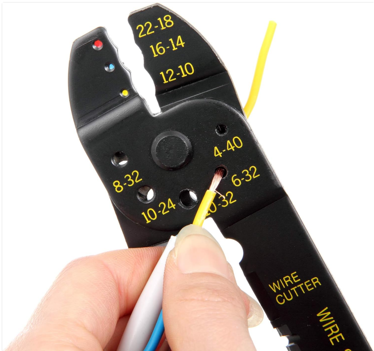
Image 5.1: A hand demonstrating the wire stripping function, inserting a yellow insulated wire into the appropriate gauge slot on the tool.
