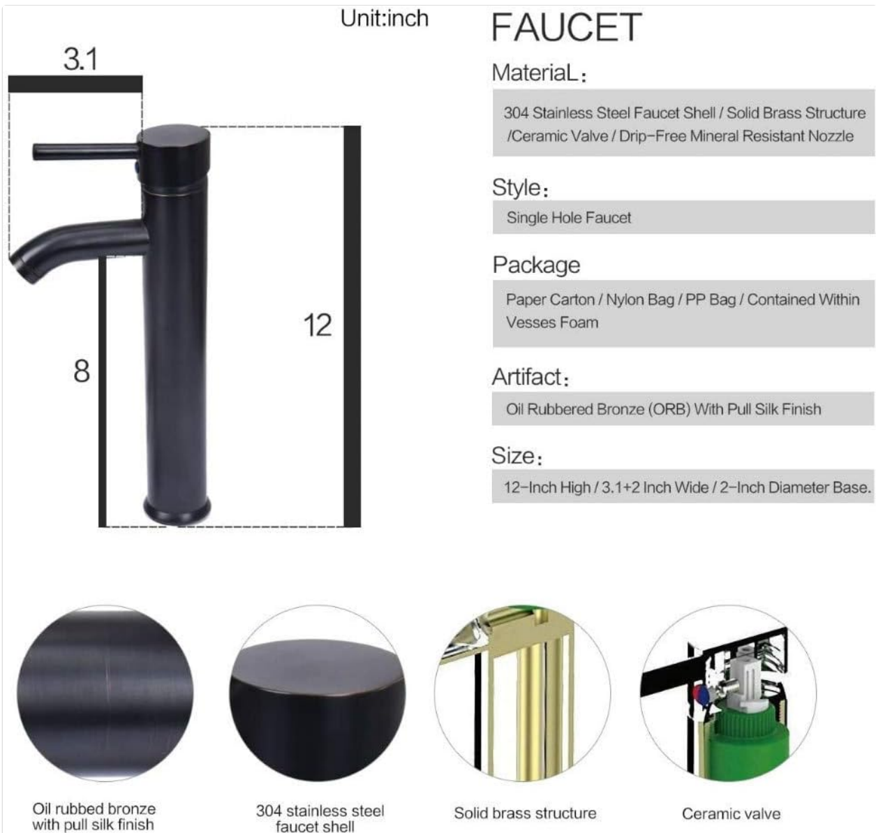
Figure 3.1: Basin and Faucet Dimensions.
