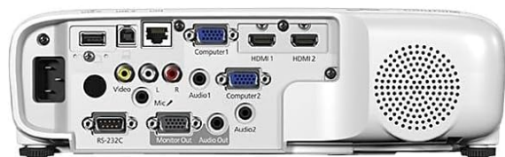
Figure 3.4: Rear Connectivity Panel. The rear panel of the projector is shown, detailing the comprehensive array of input and output ports, including HDMI, VGA, USB, Audio In/Out, Video, and LAN connections.
