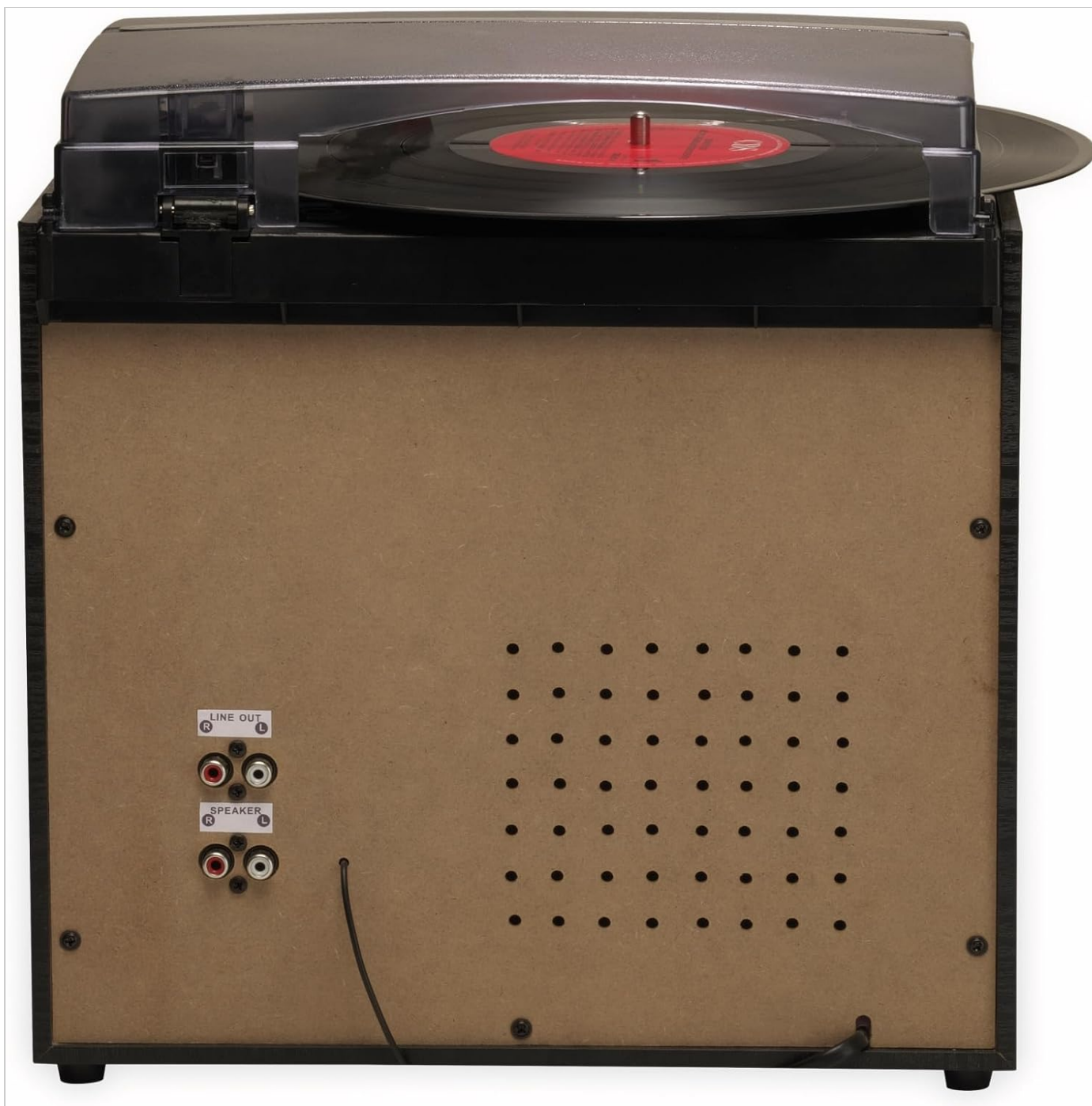
Figure 2: Rear panel of the main unit, highlighting the "LINE OUT" RCA ports and "SPEAKER" terminals for connecting external speakers. A power cable is also visible.
