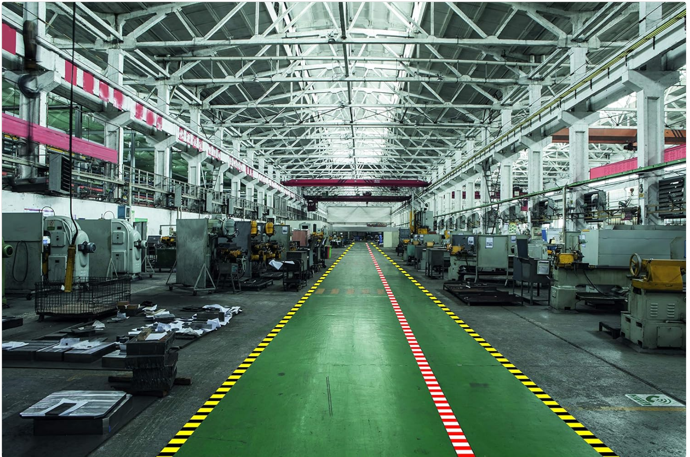
Image 2: An example of safety marking tape applied to a factory floor, illustrating its use in defining pathways and work areas.
