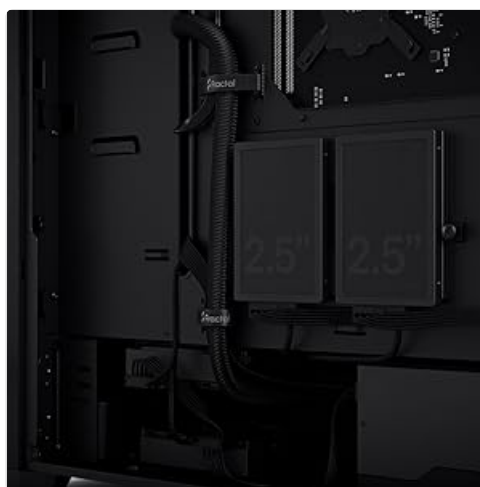
Figure 4.5: Dedicated channels and Velcro straps for efficient cable routing.
