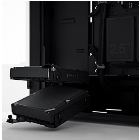
Figure 4.2: Illustrates the mounting points for 2.5" SSDs and 3.5" HDDs.
