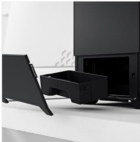
Figure 5: Close-up view of the 5.25" bay, showing the integrated storage drawer and magnetic cover.
