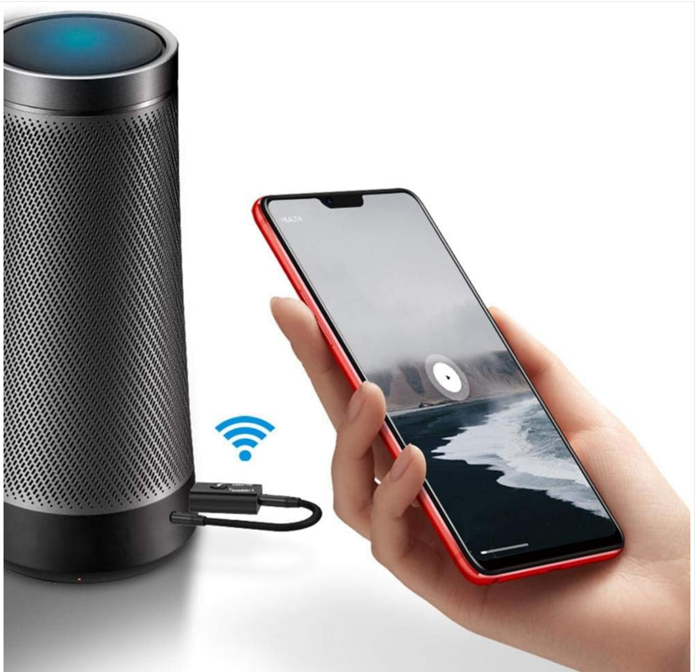
Figure 6: The device connected to a traditional wired speaker, enabling it to receive audio wirelessly from a smartphone.
