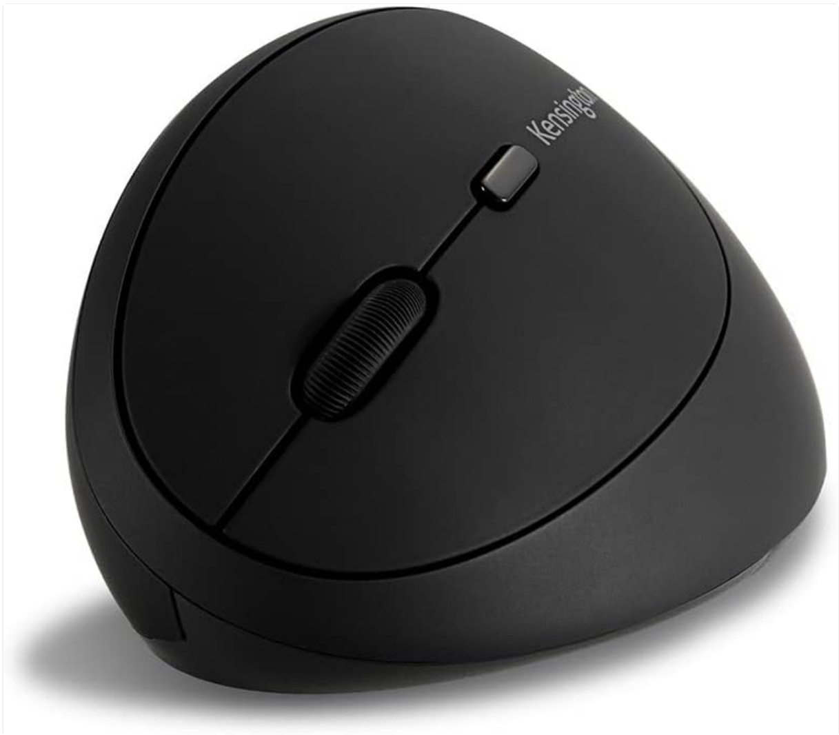
Image: Top view of the mouse, displaying the scroll wheel, left/right click buttons, and additional customizable buttons.
