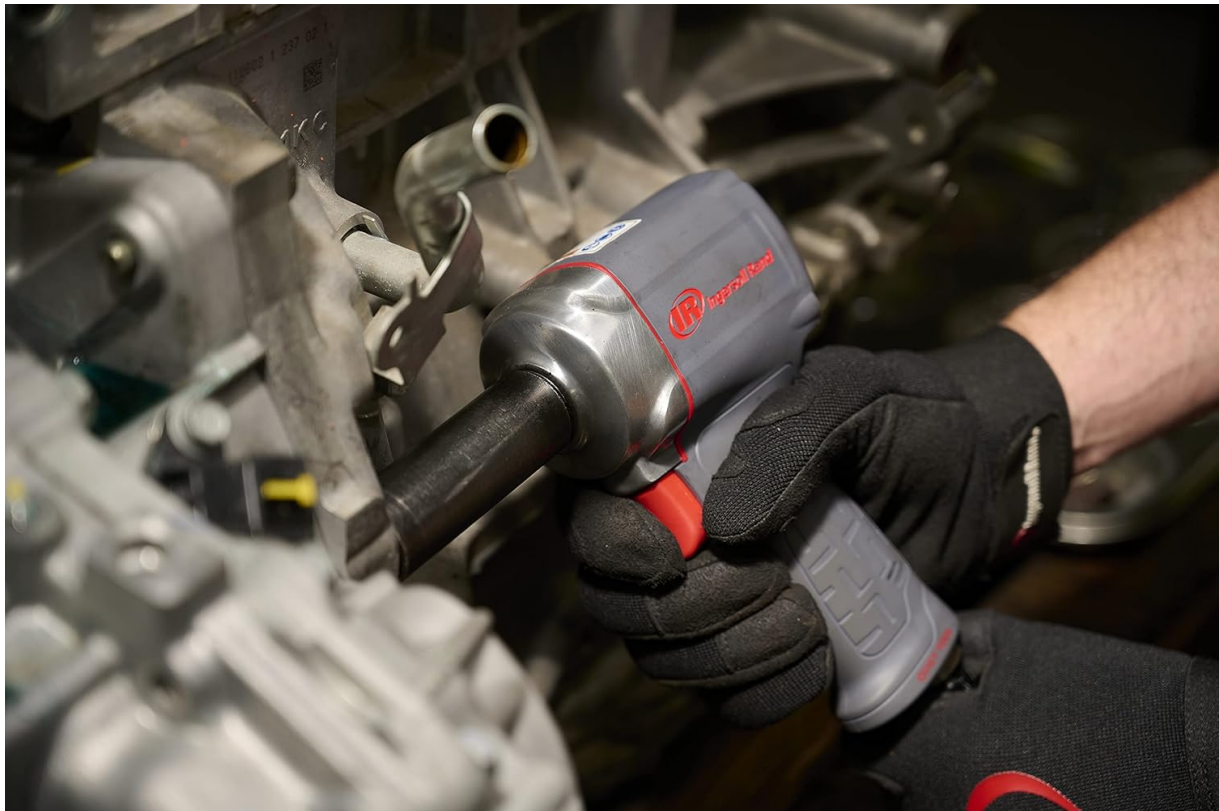
Image: The Ingersoll Rand 36QMAX impact wrench with a socket attached to its 1/2-inch square drive, demonstrating readiness for operation.
