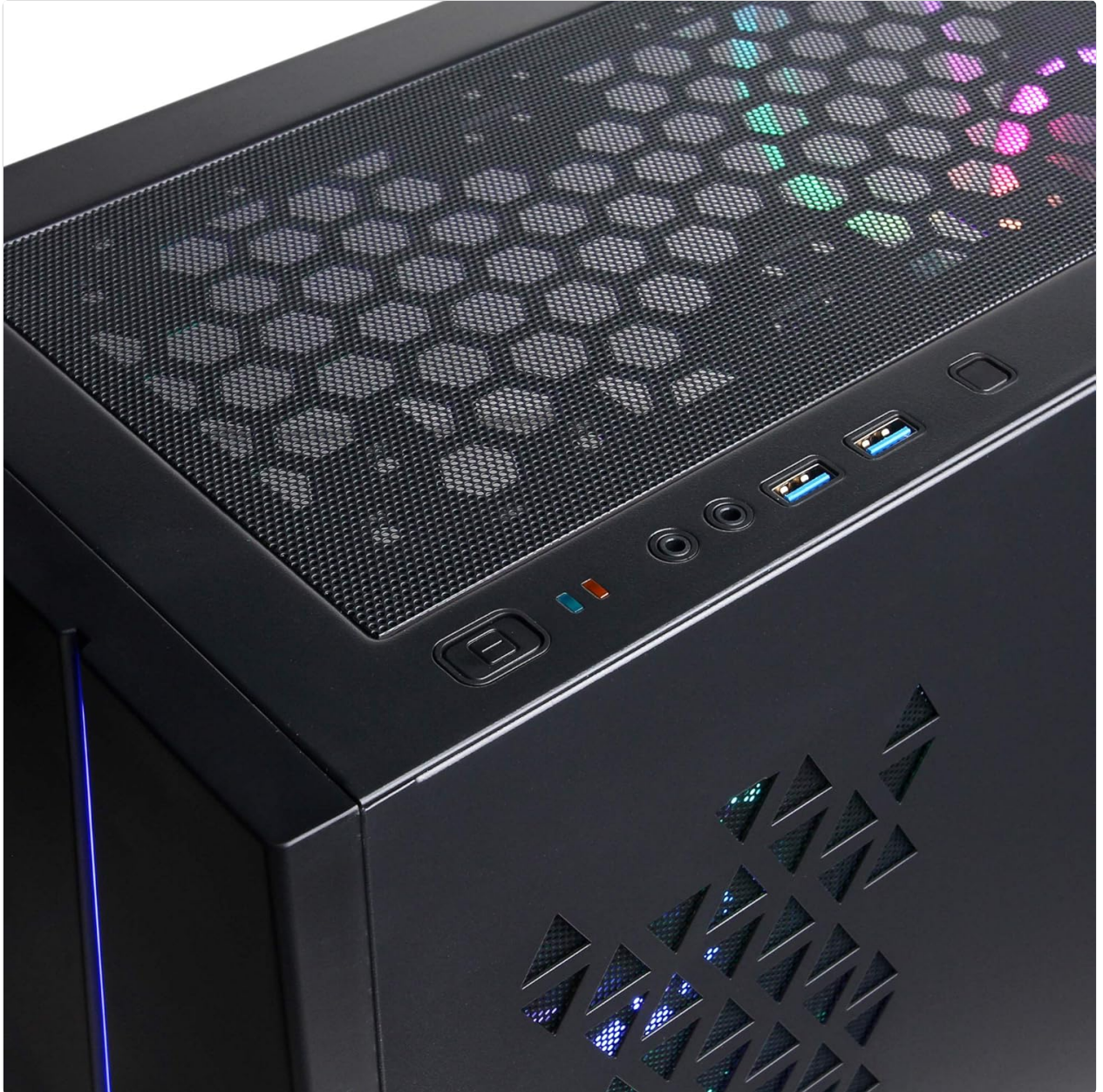
Image: A close-up view of the top panel ports, including USB and audio jacks, for convenient peripheral connection.
