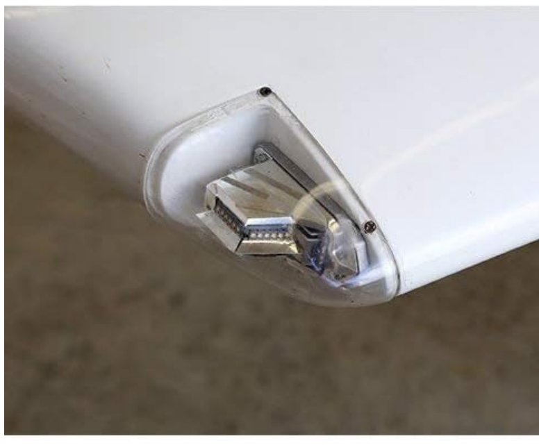
Figure 2: The Whelen Orion 650E light installed on an aircraft wingtip. This image demonstrates the flush-mounted integration of the light into the wing structure, highlighting its low-profile design.
