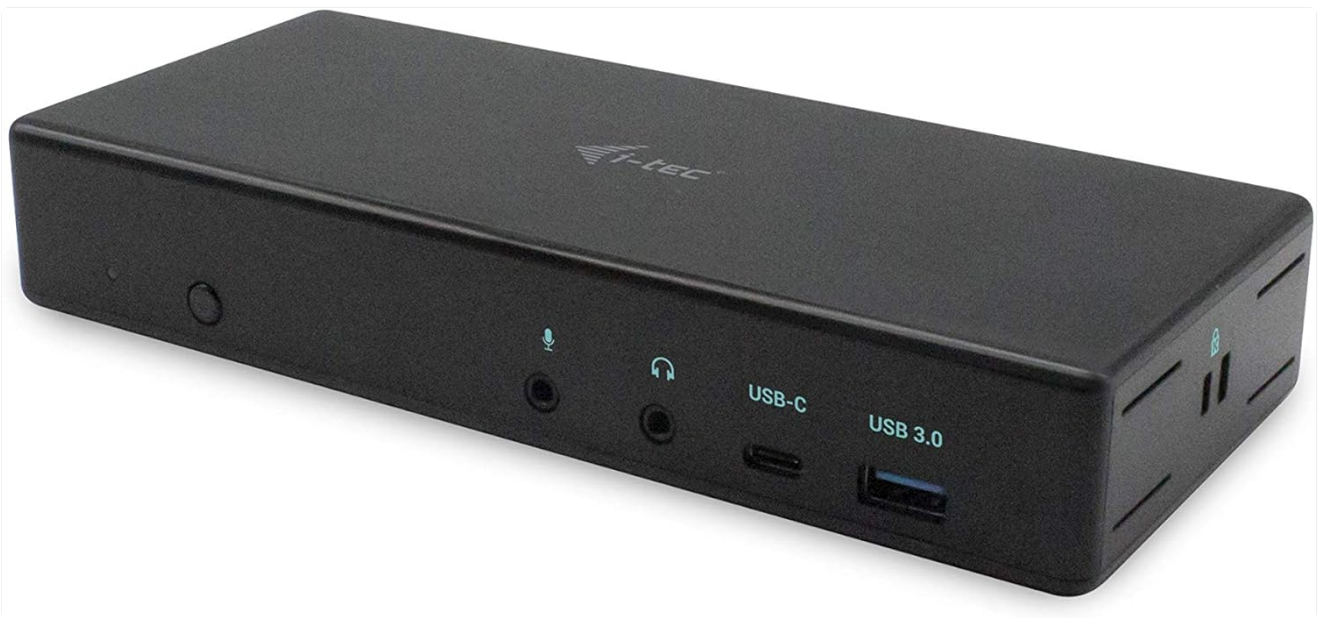
Figure 3.1: Front Panel. This image shows the front of the docking station with a power button, microphone input jack, headphone output jack, one USB-C data port, and one USB 3.0 port.
