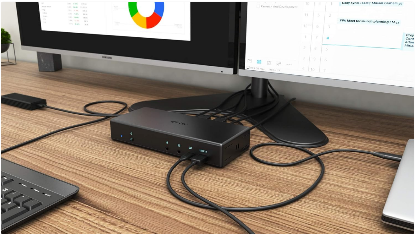
Figure 5.4: Connected Workstation. This image provides a close-up of the docking station on a desk, connected to a laptop via USB-C, and featuring various peripherals plugged into its front ports, including a USB drive and audio devices.
