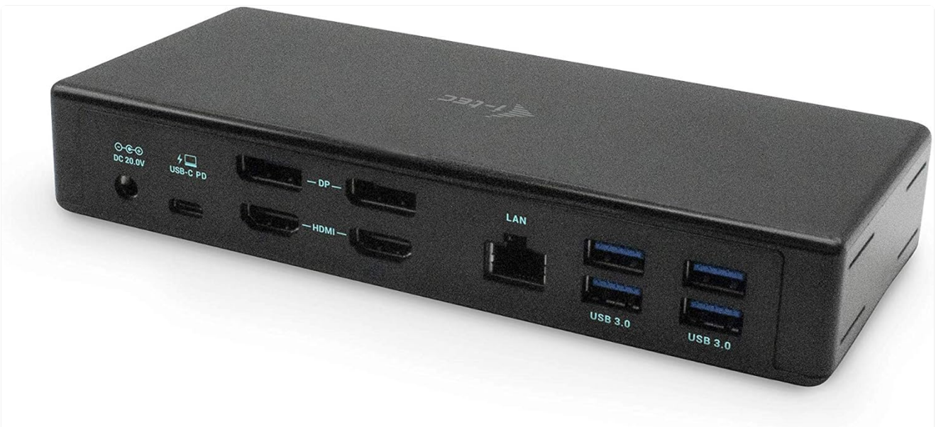
Figure 3.2: Rear Panel. This image displays the rear of the docking station, featuring the DC 20V power input, USB-C PD host connection, two DisplayPort outputs, two HDMI outputs, a Gigabit Ethernet (LAN) port, and four additional USB 3.0 ports.
