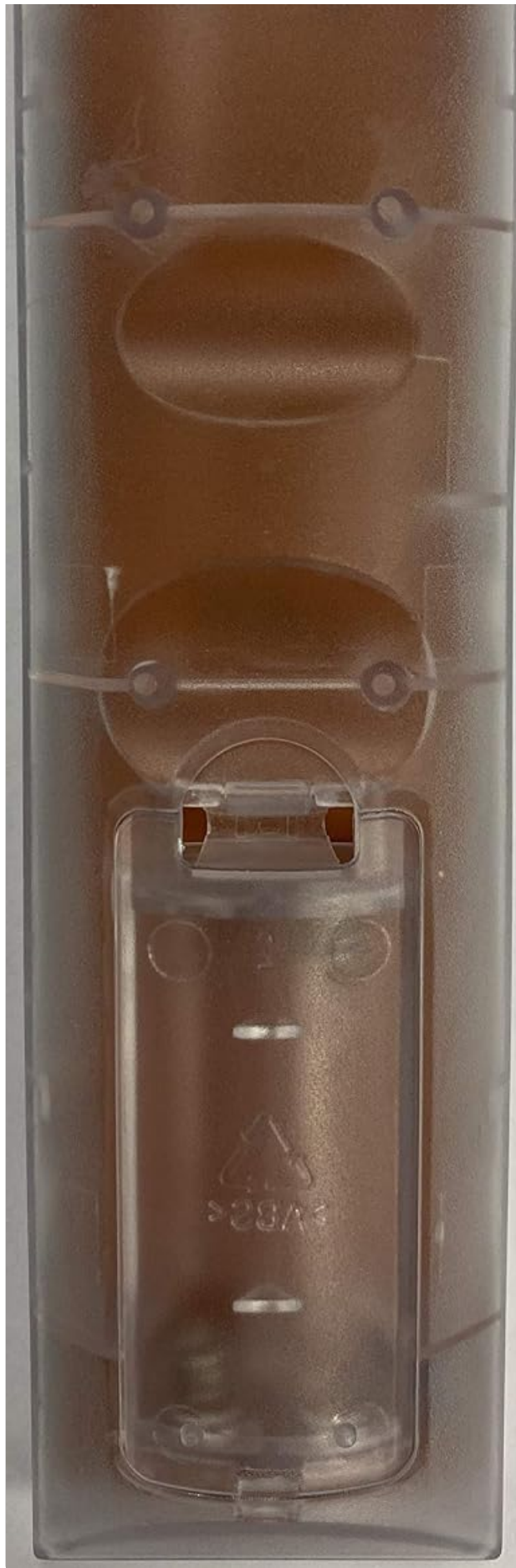
Figure 5.1: Back view of the Eden TVOEM1900 remote control. This image highlights the transparent back casing and the battery compartment cover.
