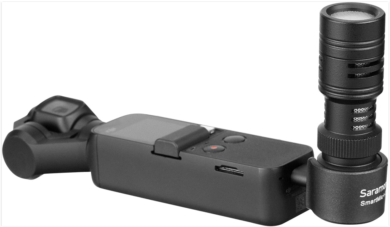
Image 3.2: The SmartMic+OP with the foam windscreen attached, mounted on the DJI Osmo Pocket.
