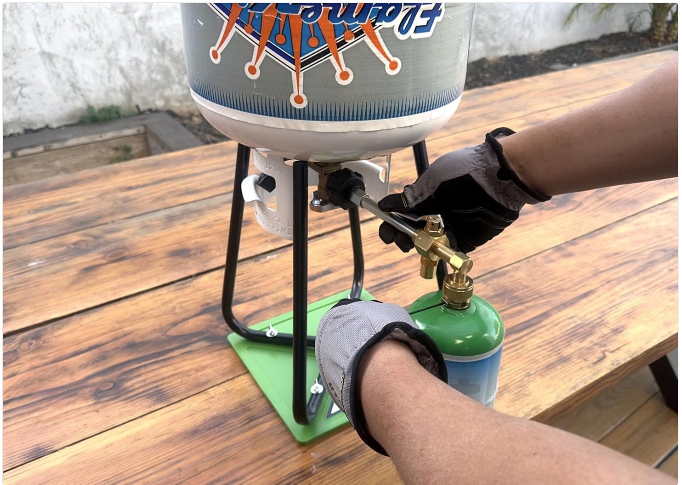
Image: The Flame King Refill Adapter Valve connected to an inverted 20LB propane tank and an upright 1LB refillable cylinder, ready for refilling.
