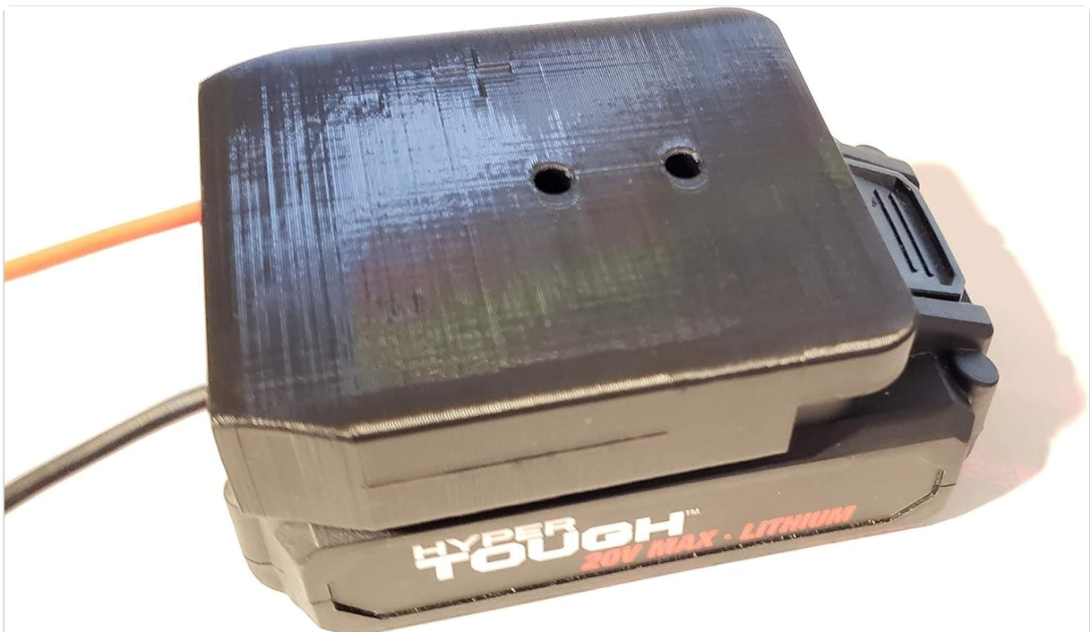
Image: The adapter securely connected to a HyperTough 20V Max Li-Ion battery. Note the positive and negative markings on the adapter.
