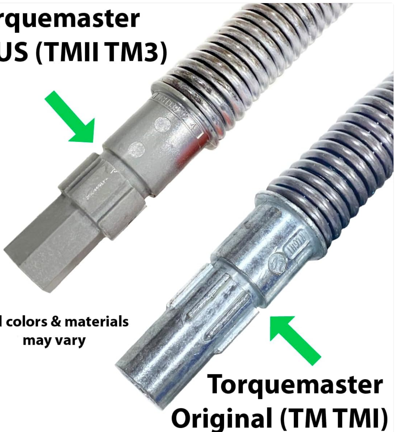
Figure 2: Visual comparison of Torquemaster Plus (left) and Original Torquemaster (right) spring winding ends. Note the hexagonal end on the Plus version and the visible counter gear on the Original.
