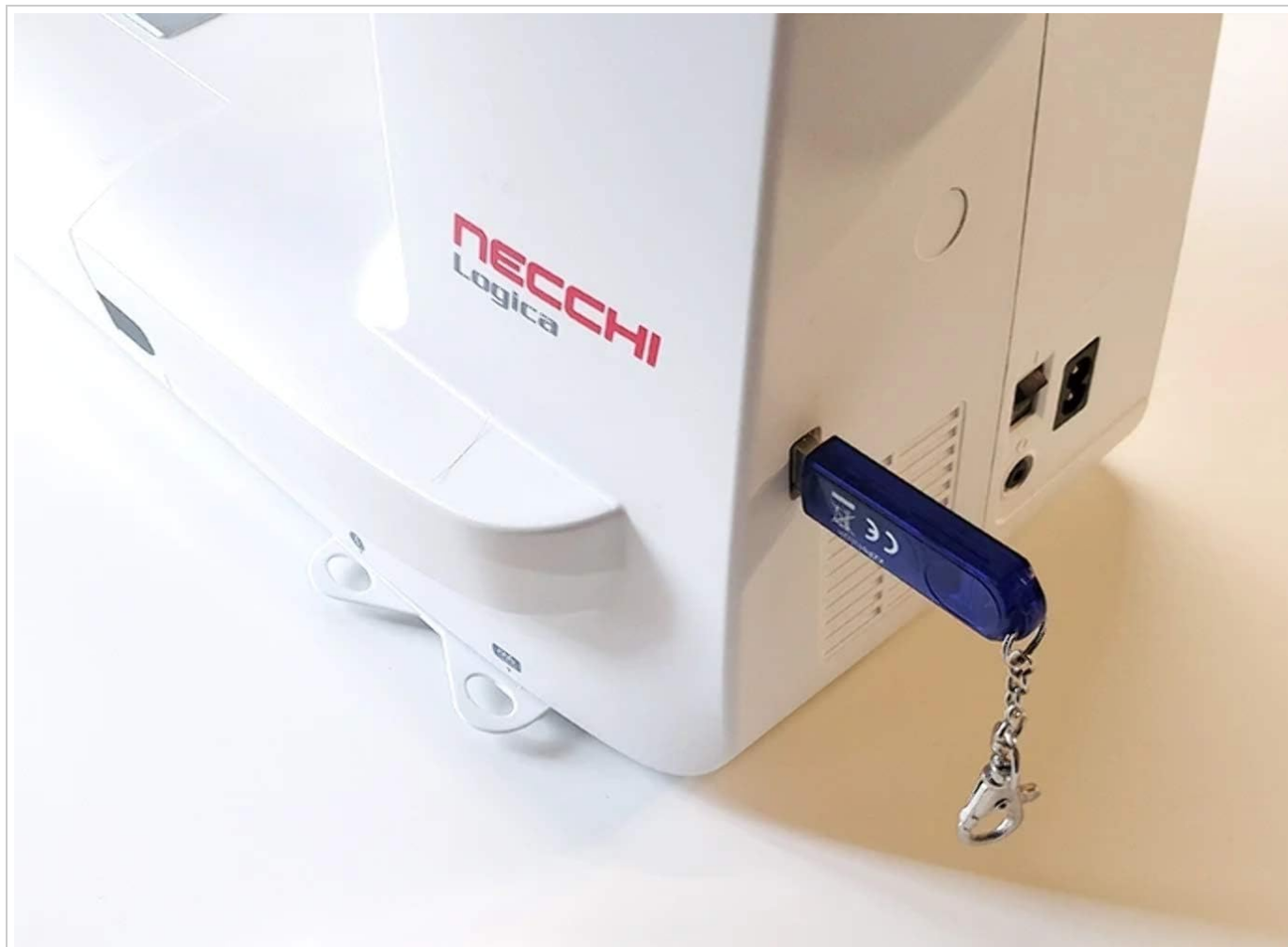
Figure 4.3: The USB port located on the side of the machine, used for transferring embroidery designs and updates.
