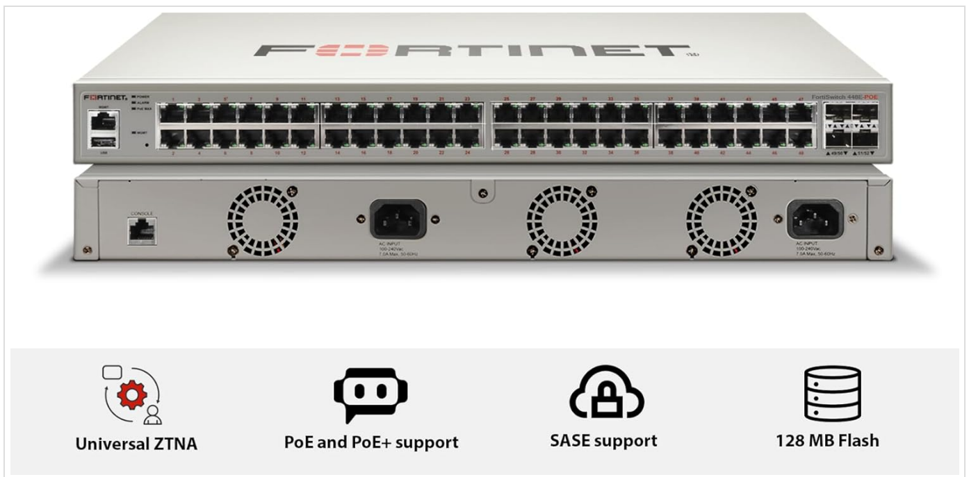
Image 3.1: Front and rear views of the FortiSwitch FS-448E-POE, showing the 48 PoE+ ports on the front and AC input, console port, and cooling fans on the rear.
