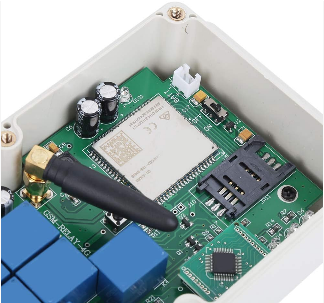
Image 2.2: Detailed view of the circuit board, highlighting the SIM card slot and the connector for the external antenna.
