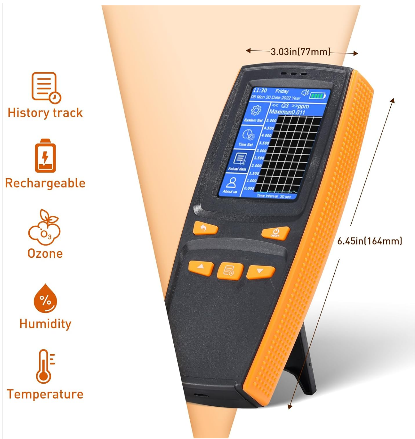
Image: The VISLONE Ozone Detector displaying its dimensions (approximately 6.45 inches in length and 3.03 inches in width) and icons representing its core functions: History track, Rechargeable battery, Ozone detection, Humidity measurement, and Temperature measurement.
