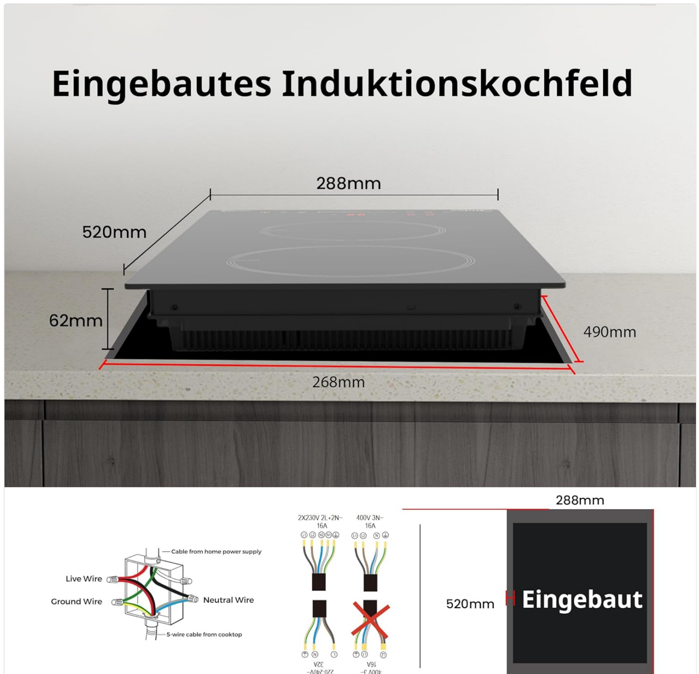
Figure 4.1: Cooktop Dimensions and Wiring Diagram. The cooktop measures 520mm (length) x 288mm (width) x 55mm (height). The cutout dimensions for built-in installation are approximately 490mm x 268mm. The wiring diagram illustrates connections for live wire, neutral wire, and ground wire to the home power supply.
