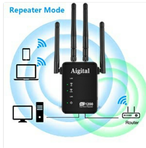
Image: Diagram illustrating Repeater Mode, where the extender receives a wireless signal from the main router and retransmits it to client devices.
