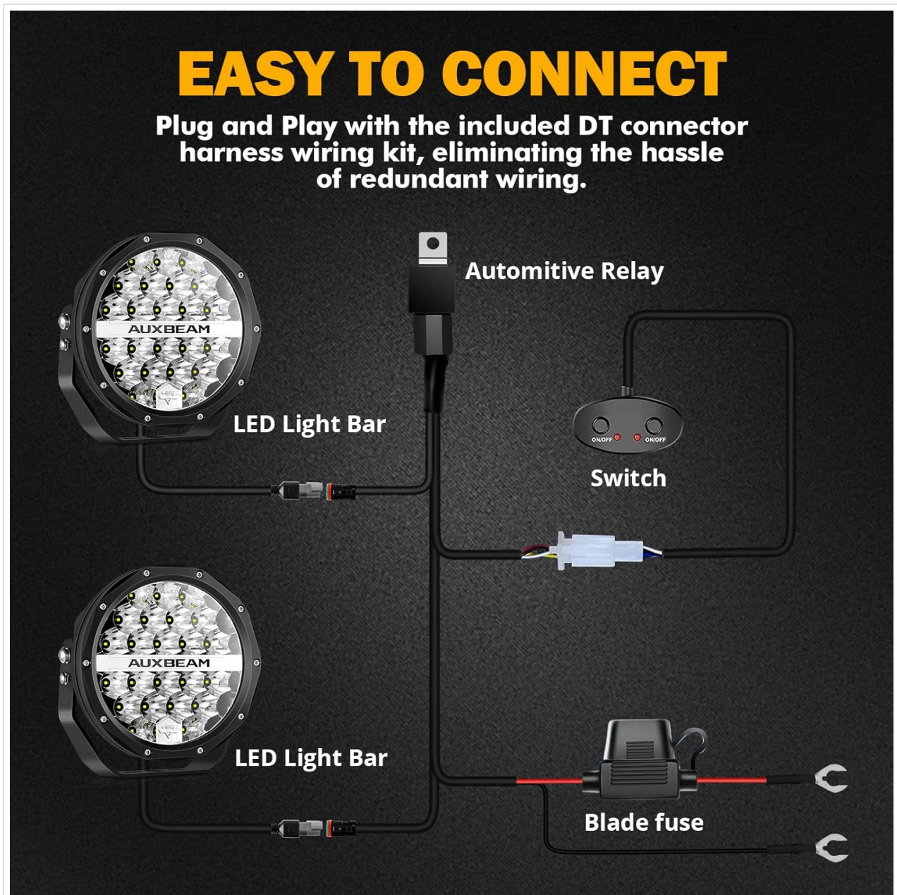
Figure 3: Detailed wiring diagram for connecting the Auxbeam LED lights.
